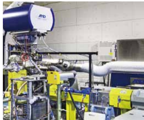
Engine bench testing system
