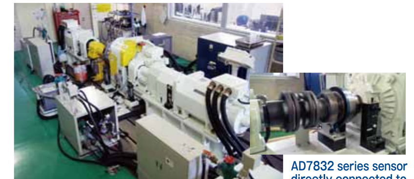
AD7832 series sensor directly connected to the load motor
