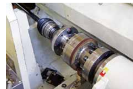
AD7832 series sensor directly connected to the drive shaft
