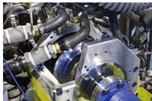
RTS sensor directly connected to engine crank shaft
