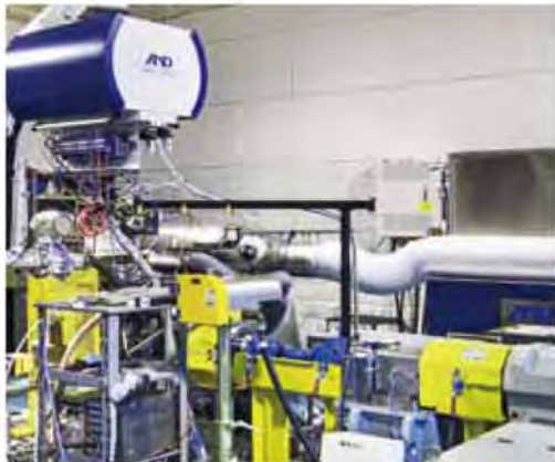
Engine bench testing system
