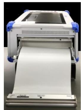
Step 5. Attach the Z-fold paper adapter to the recording paper guide of the printer cover.
