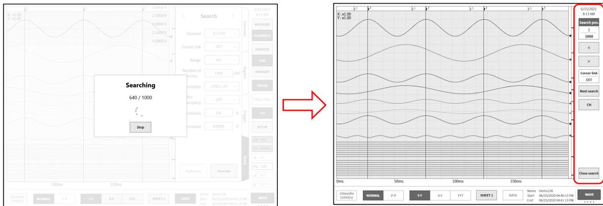
Step 6. When there are one or more search results, press the **[<]** key (back)/**[>]** key (forward) in the "7.5.10. Search Display Menu" to change the waveform display. You can press the **[CH]** key to return to the channel setup sub menu and reset the search conditions. Press the **[Close search]** key to return from the "7.5.10. Search Display Menu" to the basic [side menu](#).
