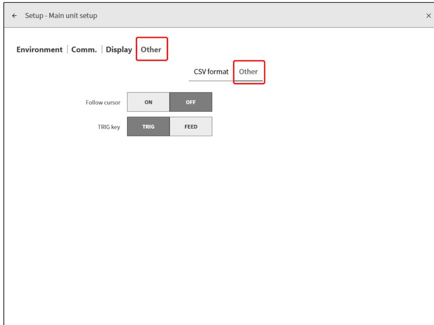
**Follow cursor:** When enabled, the waveform and cursor are displayed when the cursor moves outside the waveform monitor. When disabled, the cursor moves but the waveform does not when the waveform moves outside the waveform monitor. (The cursor line will no longer be displayed.)
