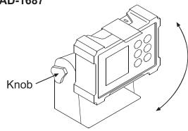
Step 1. Loosen the knob and adjust the angle of the AD-1687 for appropriate viewing.
