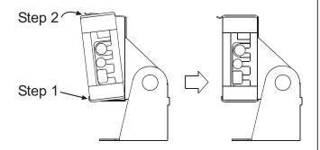
Step1. Insert the bottom of the AD-1687 into the lower part of the stand.
