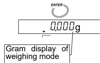
To cancel the new parameters and return to the weighing mode, press the **RESET** key.
