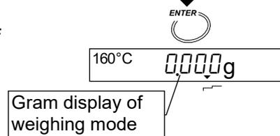
To cancel new parameters and return to weighing mode, press the **RESET** key.
