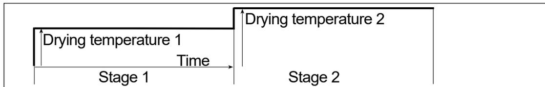
"Temperature 1" can be set higher than "temperature 2" in step drying.
