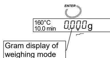
To cancel the new parameters and return to the weighing mode, press the **RESET** key.
