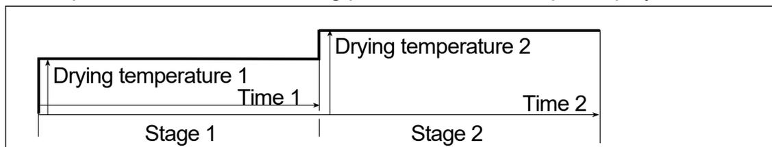
"Temperature 1" can be set higher than "temperature 2" in step drying.
