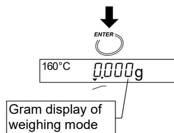
To cancel the new parameters and return to the weighing mode, press the **RESET** key.
