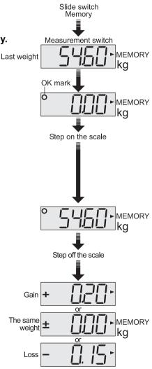
Displaying the Weight Data Stored in the Scale
