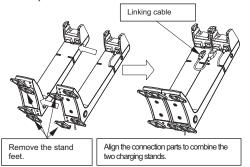
Attach the stand feet to link the two charging stands, with the front foot and the rear foot facing opposite directions
