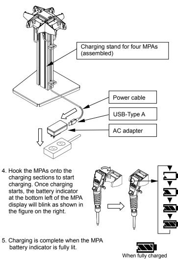
6. The MPAs can continue to be hooked to the charging stand after they are fully charged. (They will not be overcharged.)
