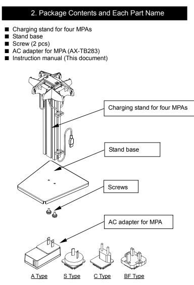
\* The A-type plug is initially attached to the AC adapter for use in Japan. For use outside of Japan, please change it to the type appropriate for your country.
