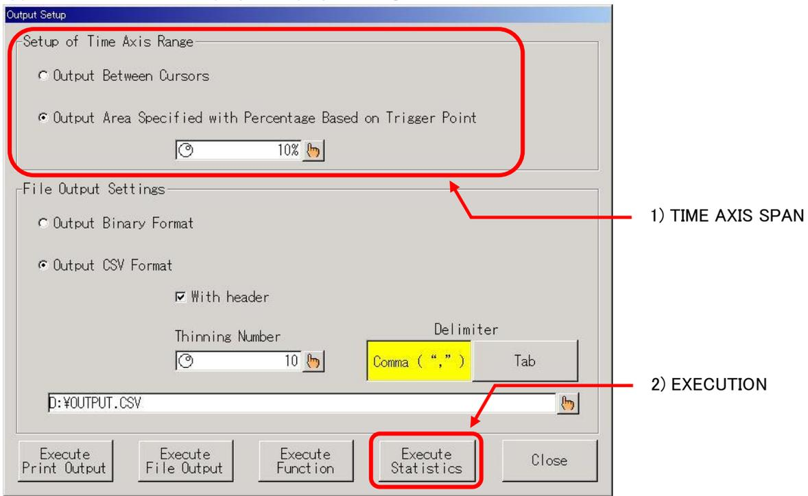
1) Time axis span setting
