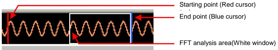
The starting point is designated by using red cursor1 on the Y-T DISPLAY, and it is also set by touching thumbnail image. Ending point is primarily determined, depending on both data length and averaging number. The white window shows the FFT analysis proceeding. The FFT analysis has already completed in the area from the red cursor to the left edge of the white window, while it is just getting underway in the white window.
