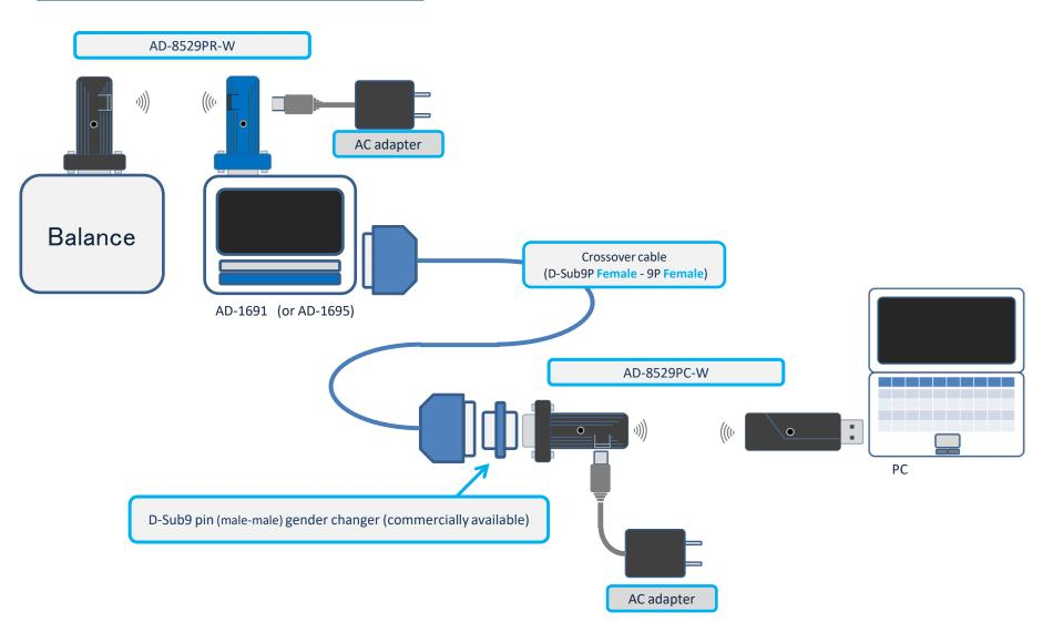
Custom cable can also be created (30 cm, for connection without using a gender changer).
