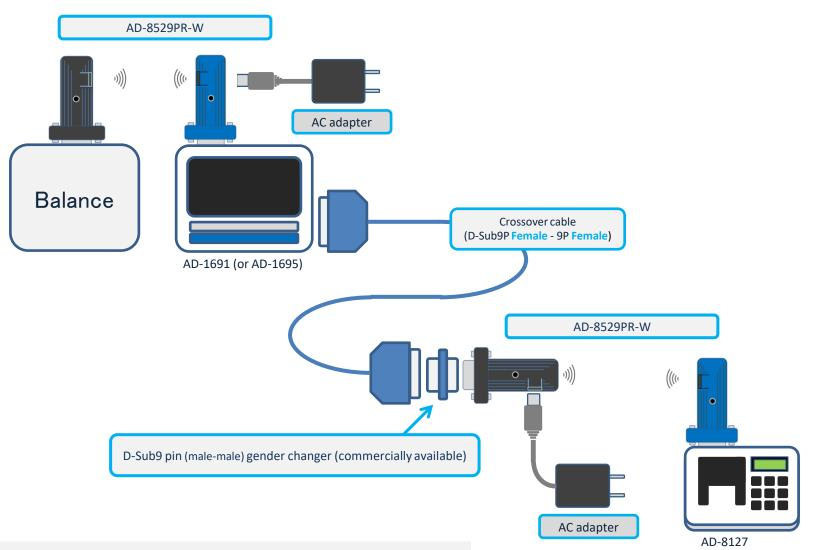
Custom cable can also be created (30 cm, for connection without using a gender changer).
