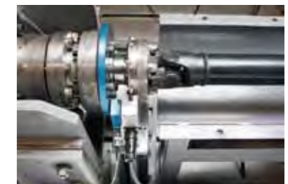
Example of attachment of dynamo intermediate axis
