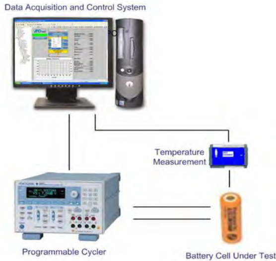
Figure 3. Battery Test Setup.
